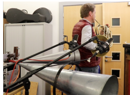
Figures 1 and 2. Experiments with the positioning the horn bell towards the recording funnels.
