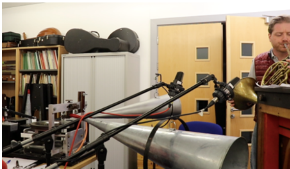
Figures 1 and 2. Experiments with the positioning the horn bell towards the recording funnels.
